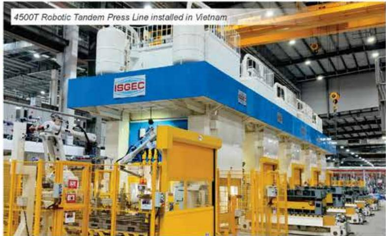
4500T Robotic Tandem Press Line installed in Vietnam
