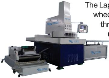
The Lapmaster Wolters DSG series of twin-wheel grinding machines are driven by three variable-speed motors for maximum process control flexibility. All three rotating machine components, the sun gear, top plate, and bottom plate, are independently controlled. Process down pressure requirements are pneumatically regulated and continuously monitored by a load cell.
