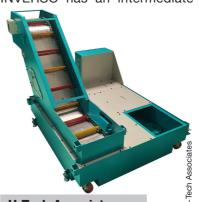
**U-Tech Associates** www.u-techindia.com Hall & Stall: 5/B-120 platform for chips to settle down – even the floating chips – which are then scraped by the scrapers. Coolant flows down and escapes into the coolant tank. Any fine dust or chips that go to the bottom of the conveyor are removed by the scrapers while moving in the opposite direction.
