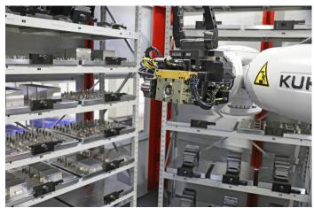
At BAM, automation encompasses all processes, from order entry through to production. In this image, a robot supplies the 5-axis machining center with pre-fitted workpiece pallets.
