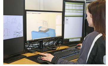
The CAM office is an essential place. Using the *hyperMILL*® high-end CAM system from OPEN MIND, employees create NC programs based on 3D design data; in some cases, the programs are even generated fully automatically.
